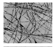
Lightly Loaded Air Entering Side Close-up photo shows open weave pattern that allows over-spray to penetrate deep into the pad.
